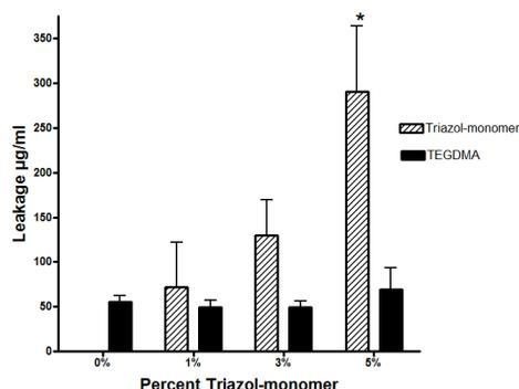
Figure 2. Leakage of unreacted TEGDMA and Triazole-monomer in a mixture of 75/25 ethanol/water (vol/vol) measured after 24h with gas-chromatography.
