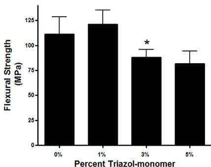
Figure 1. Flexural strength was measured with three point bending according to ISO 4049.
